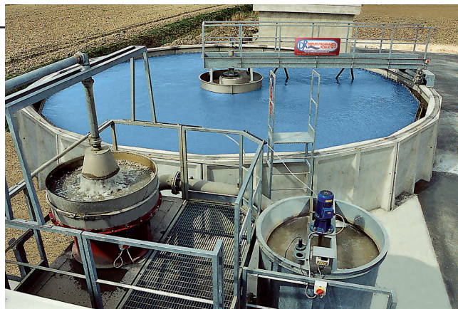
Water treatment/recycling system with 60-70 m³/h capacity, ancillary to polypropylene big-bags and LDPE film recycling line 1000-1200 kg/h
