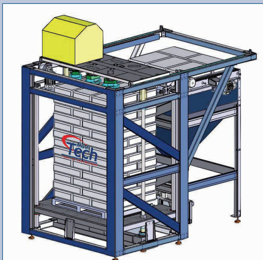
Rendering of a bag depalletising, cutting and emptying system exhibited by Main Tech at K 2013
