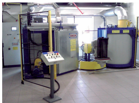
A Rotaut RT1051B machine, with an offset arm, a digital burner for LPG, and an Omron PLC, has been recently supplied by Caccia Engineering to a big Belgian multinational company
