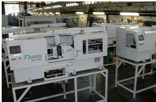
The new Presmall SC 6 distinguishes itself from the previous model mainly for the 6-ton tiebarless clamping unit and the multi-axis control system driving up to 16 axes
