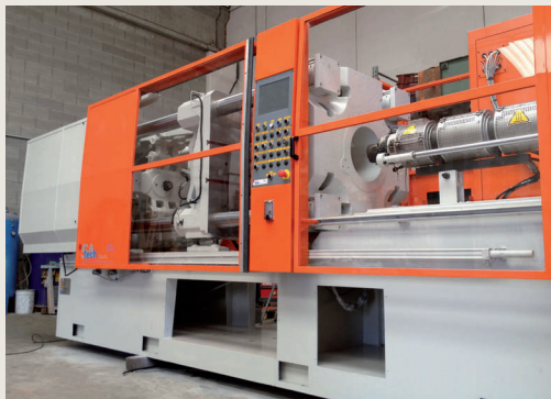
A 400-ton RMP injection moulding machine after SA Tech's global reconditioning
