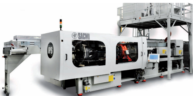
At the Sacmi stand a pivotal role is played by the IPS 220 B, a new-concept injection preform press
