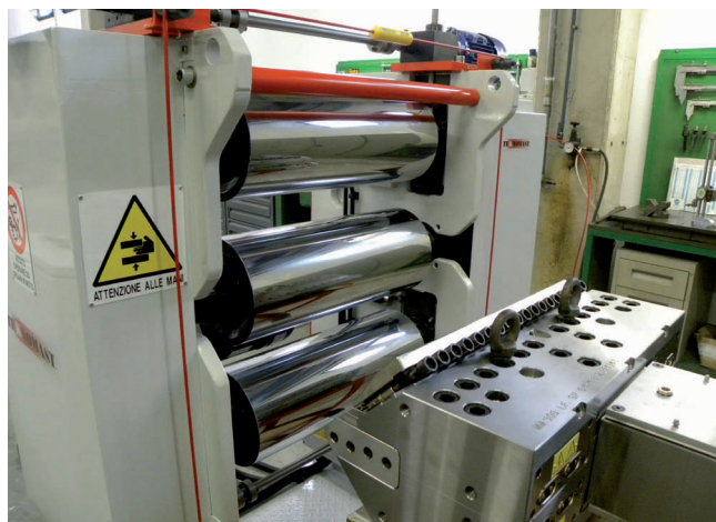
Teknomast has a very diverse range of calenders, with a table from 400 to 2,500 mm and a diameter from 200 to 600 mm
