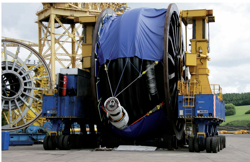
Giant flexible pipes made from the polyamide 12 Vestamid NRG by Evonik
