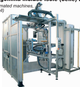
Isole (celle) robotizzate soffietto posteriore, anteriore e portiere auto Robotized island (cell) rear bellows, front bellows, car door bellows
