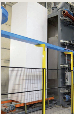
Block moulder with new waterless vacuum system
